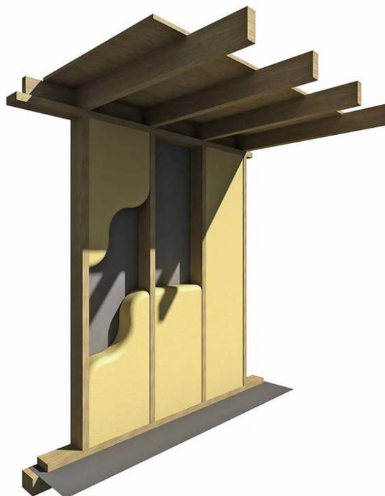
Figure 10: Raccord sol plafond
